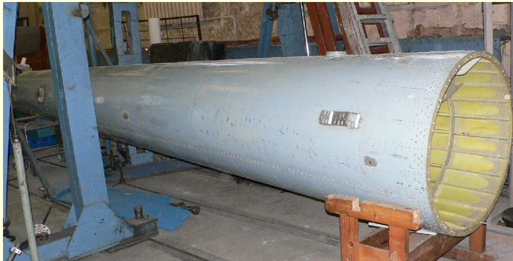
Figure 1. Common view of the MI8 helicopter tail beam before mounting for full-scale fatigue testing
